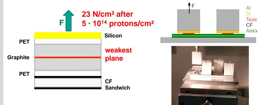
Irradiation of 5.10<sup>14</sup> protons/cm<sup>2</sup> reduces strength by about 40% (23 N/cm<sup>2</sup>)
