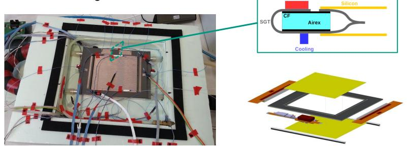
With SGT complex cooling structures can be realized very easily due to its flexibility
